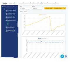
Graph of tank filling. Depth of storage is not limited. According to the accumulated data, reports are available in tabular and graphical form. Downloading data to Excel, PDF, CSV, JPG, PNG is available.
