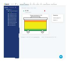
Intuitive dispatcher interface. Displays the level of filling of containers, in individual and group representation, in the form of text and mnemonic diagrams.
